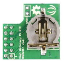
The High Accuracy Pi RTC is based on the clock chip DS3231. The DS3231 is a lowcost, extremely accurate I2C realtime clock (RTC). It provides an RTC for Raspberry Pi via the I2C interface. The RTC maintains seconds, minutes, hours, day, date, month, and year information.
