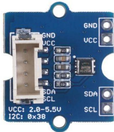
AHT20 is a new generation of temperature and humidity sensor embedded with a dual-row flat and no-lead SMD package, suitable for the reflow soldering. AHT20 is equipped with a newly designed ASIC chip: an improved MEMS semiconductor capacitive humidity sensor, and a standard on-chip temperature sensor. The output is the I2C protocol with the Grove interface.
