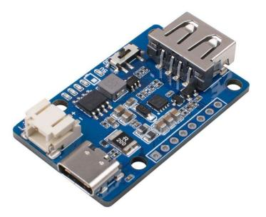
The Lipo Rider Plus from Seeed is not only a **Fast Charger** but also a **Strong PowerBoost**, supports up to 5V/2A charging current, boost output integration, output up to 5V/2.4A, can also output 3.3V /250mA.
