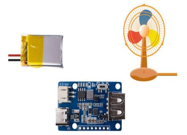
Not only a charger but also a power supply and a booster. With the help of Lipo Rider Plus, you can input a 3.7V lipo battery, and output up to 5V/2.4A via the USB Type-A port. With the on-board switch, you can control the ON/OFF of USB port easily. Meanwhile, we provide the full function pin header, which can output 3.3V/250mA as well.
