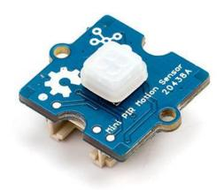
PIR sensor is used for making motion detecting applications such as alarm burglar systems, visitor presence monitoring, light switches and robots.
