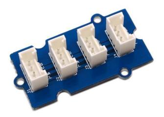
I2C Hub Grove is an extension Grove module for connecting multiply I2C devices to Grove Base Shield
