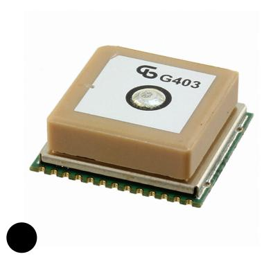
The A2235-H GPS module enables fast acquisition and tracking with SiRFstar IV technology. This small form-factor module addresses the demand for low power consumption with SiRFaware technology. The removal of jammers and high sensitivity during acquisition allows for use in many different environments and under tough operating conditions.
