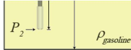
The atmospheric pressure  $P_0$  on the liquid surface is introduced into the back chamber of the sensor through the air guiding tube to offset the atmospheric pressure  $P_0$  at the end of the sensor, so that the measured pressure of the sensor is  $P' = P - P_0 = \rho gh$ . Therefore, if the **liquid density  $\rho$**  and the **acceleration of gravity  $g$**  are known, the liquid level depth  $h$  can be calculated by measuring the pressure  $P'$ .
