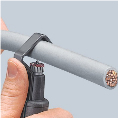
Setting the tool for circular cut
