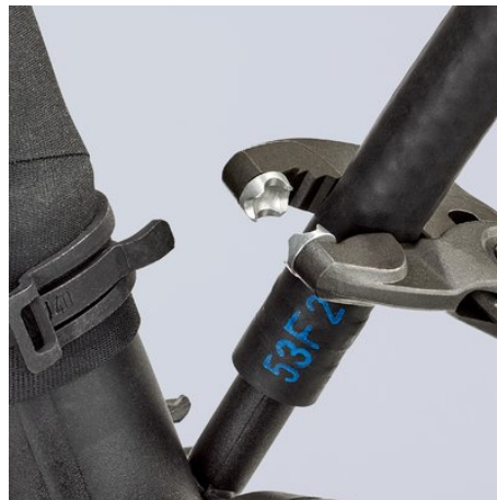
additional function: detach hoses gently using the serrated jaw
