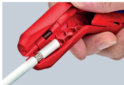
Dismantling of a coax cable
