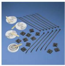
EMA Epoxy supplied in convenient two-compartment mixer cup with a mixer stick for each cup. Each cup contains adhesive for three (3) EMA or ASMS mounts. Epoxy hardens in about five (5) minutes. Supports about 5 lbs. after first 15 minutes. After full 24 hour curing time, bonding strength will exceed 50 lbs. on clean, grease-free surface. EMSK3-1-X0 is an Epoxy Kit with mounts. EMSK-12-4-12-X0 is an Epoxy Kit with mounts and cable ties packed in a sturdy foil pouch.
