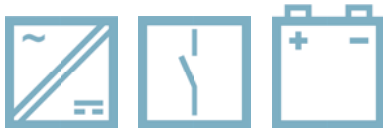
Power supply UPS module Energy storage devices
