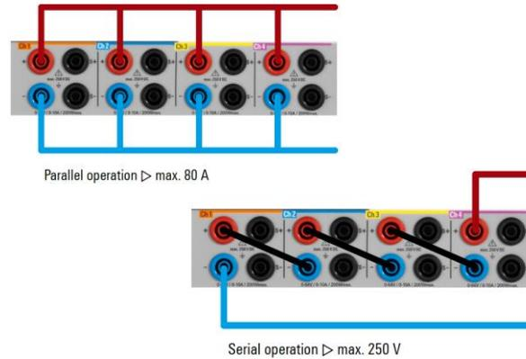
For applications requiring more voltage or current, the outputs can be connected in series or parallel to attain up to 250 V (R&S®NGP824) or 80 A (R&S®NGP804). When using the tracking function, the voltage and current are simultaneously adjusted on all selected channels.
