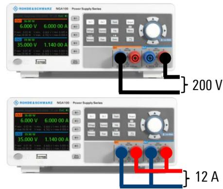
Activate channel fusion in either serial or parallel mode and the device will act like a single-channel version of itself. In serial mode, the outputs are connected internally, while the parallel mode requires external wiring.
