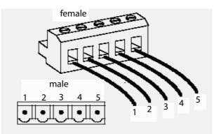
Color stickers that match communication cable colors are attached to the communications connectors. Match the colors when connecting communication cables to the connectors, the colors can be found in the next table.
