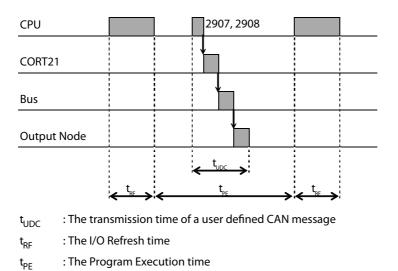
After the content of the message command is transferred to the User Defined CAN Unit, the unit immediately relays the contained message to the CAN transmission interface. The actual transmission delay of the message depends on the bus load and the message priority (identifier). Refer to 5-1-4 CAN Interface for the message delay time on the bus. The time required for an output to be set or a value in the Output Node to be changed depends on the characteristics of the Output node.
