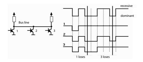
The priority at which a message is transmitted compared with another less urgent message is specified by the identifier of the message concerned. The priorities are defined during system design in the form of corresponding binary values and cannot be changed dynamically. The identifier with the lowest binary number has the highest priority.
