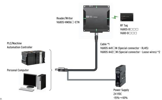
The cable can be extended up to 60 m by using the Extension Cable V680S-A40□M (cable length: 10/20/50 m). Use the extension cable between the Reader/Writer and cable.
