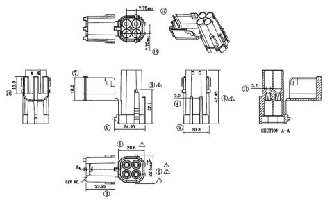
4 Pole Pin Type Female Housing for Weather Pack
