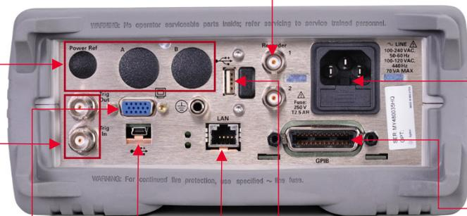
Line power accepts voltage with automatic range selection
