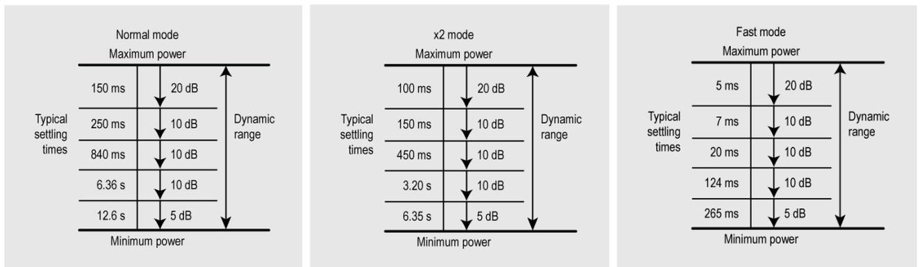
Figure 8. Auto-filter, default resolution, 10 dB decreasing power step
