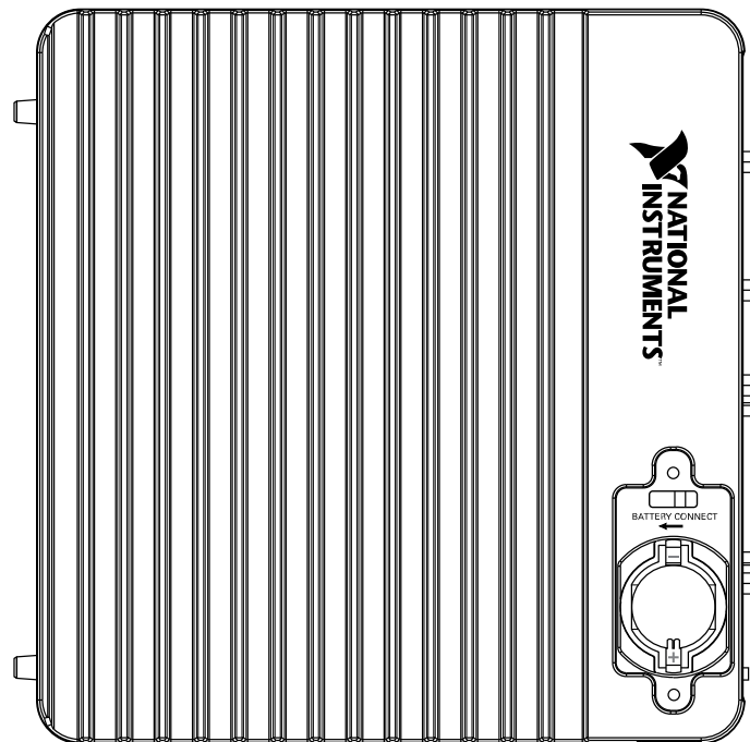
Figure 18. Side of Device with Removed Battery Cover Plate and BATTERY CONNECT Switch in Disconnected Position
