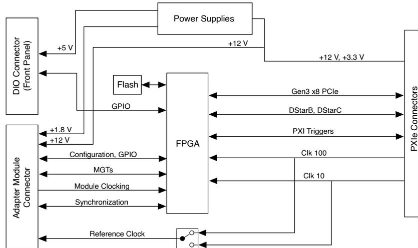
The following figure shows a block diagram of the carrier portion of the PXIe-5745 (KU040 and KU060 FPGA options).
