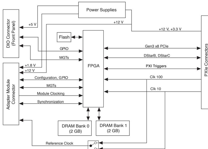
The following figure shows a block diagram of the I/O portion of the PXIe-5745.
