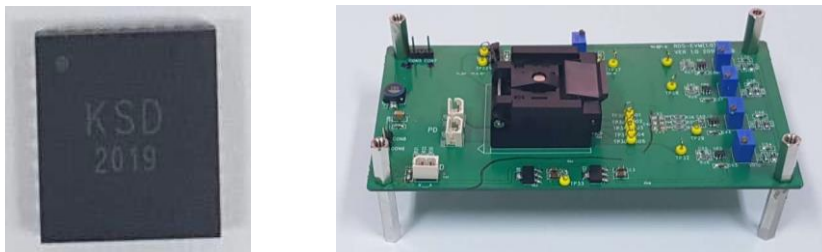
Figure 2. 2 nd generation PCIC (QFN – 32 pins 5mm x 5mm) and its test board
