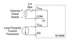
Connecting a Three-Wire Current Transducer
