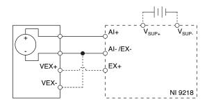
The NI 9218 provides optional 12 V sensor excitation. To use the 12 V excitation, connect a 9 VDC to 30 VDC power supply to Vsup, connect the excitation terminals on your sensor to EX+/EX-, and enable 12 V excitation in your software.
