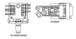
Pins 3a and 3b are tied together on the NI 9982.
