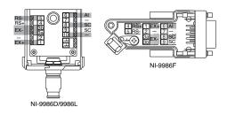
Pins 3a and 3b are tied together on the NI 9986.
