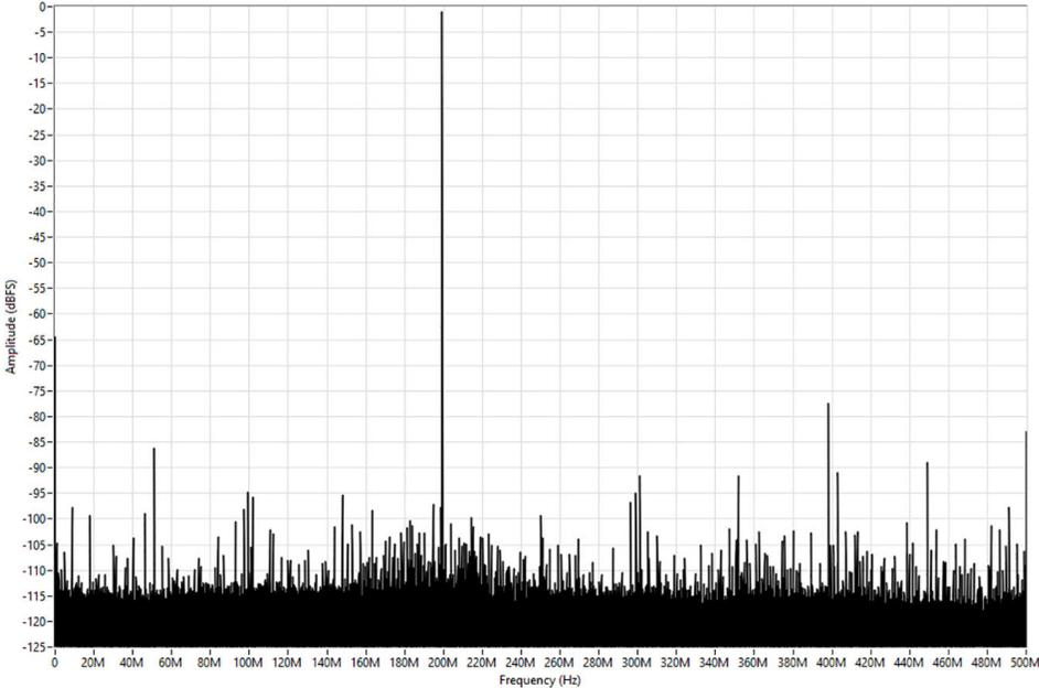
**Channel-to-channel crosstalk AC-coupled, measured**
