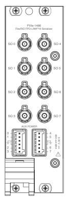
Figure 3. PXIe-1486 SerDes Front Panel
