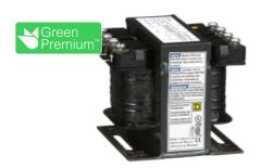
Industrial control transformer, Type T, 1 phase, 75VA, 240x480V primary, 120V secondary, 50/60Hz
