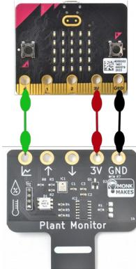
As before, power is supplied by the micro:bit, but this time, micro:Bit pin 0 is used to connect to the analog output of the Plant Monitor.
