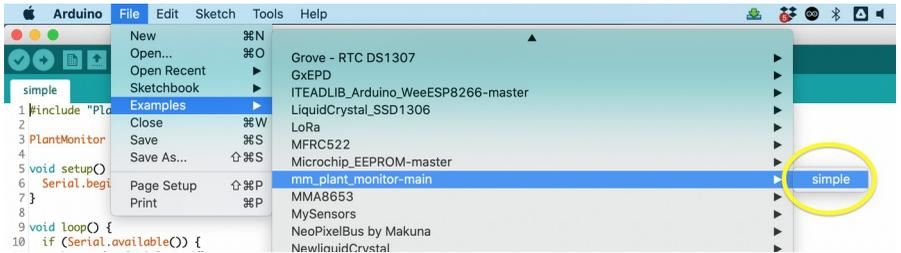
Upload the example called *Simple* to your Arduino and then open the Serial Monitor. Here, you will see a series of readings. You can also turn the Plant Monitor's LED on and off from the Serial Monitor by sending serial commands. Type L in the send area of the Serial Monitor and then press the Send button to turn the LED on, and l (lower-case L) to turn the LED off.
