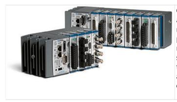
CompactRIO combines an open-embedded architecture with small size, extreme ruggedness, and C Series modules in a platform powered by the NI LabVIEW reconfigurable I/O (RIO) architecture. Each system contains an FPGA for custom timing, triggering, and processing with a wide array of available modular I/O to meet any embedded application requirement.
