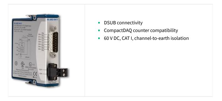
The NI-9411 works with industrial logic levels and signals for direct connection to a wide array of industrial switches, transducers, and devices. The NI-9411 is a correlated digital module, so it can perform correlated measurements, triggering, and synchronization when installed in a CompactDAQ chassis.
