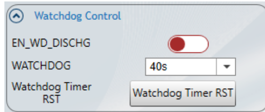
Figure 21: I 2 C Watchdog Timer Setting
