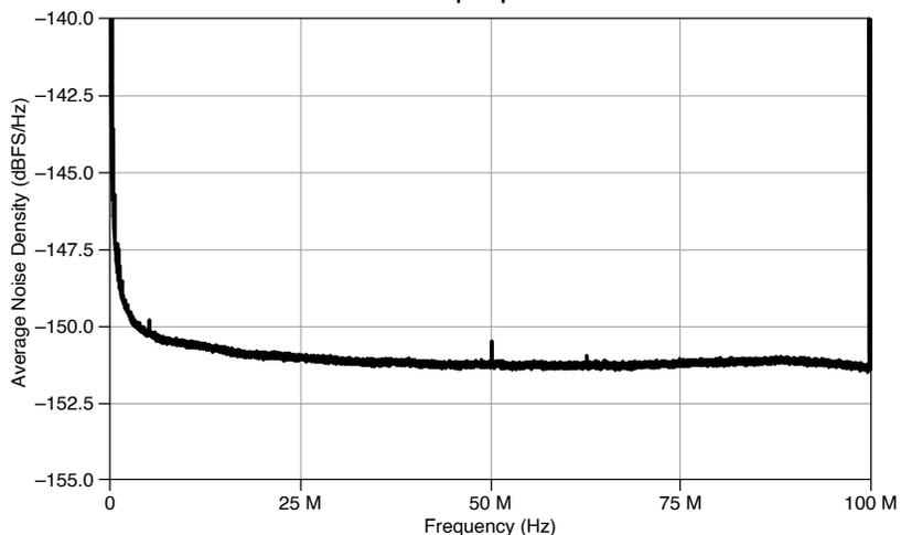
Figure 6. 50  $\Omega$  Average Noise Density, 0.2 V<sub>pk-pk</sub> Range, Measured
