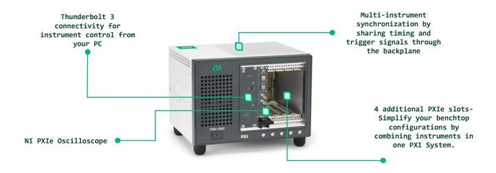
With the PXI Oscilloscope, acquire and analyze time- and frequency- domain analog signals. The PXI Oscilloscope Bundles feature up to 8 channels that can sample at speeds up to 5 GS/s with 1.5 GHz of analog bandwidth.
