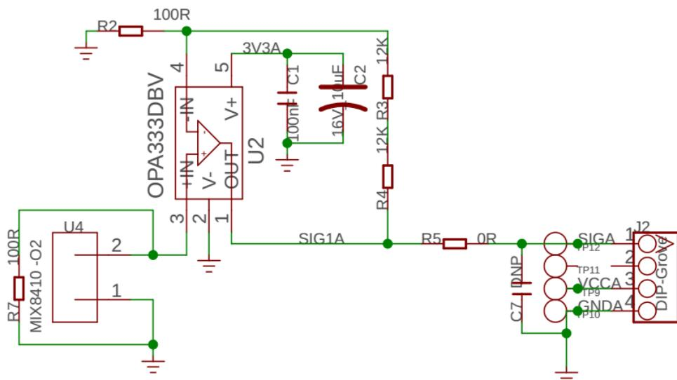
The gain of the amplifier is 241, SIGA voltage is 241 times of label #3 point voltage.
