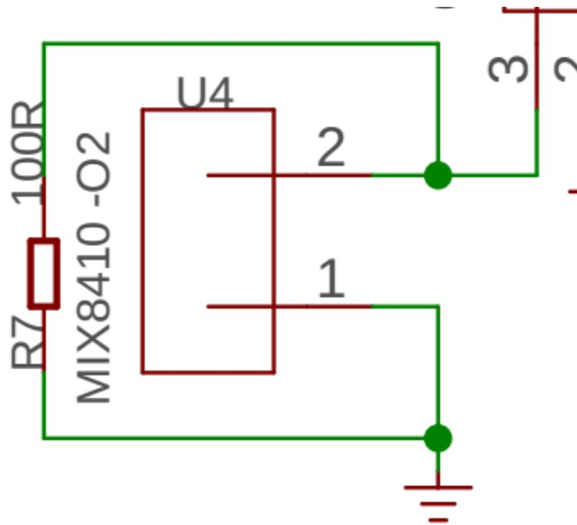
The MIX8410-O2 is current source. The voltage of the label #3 point is  $R7 * \text{Current}(\text{MIX8410-O2})$ .
