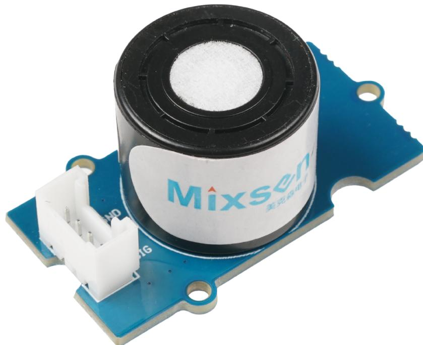
Grove - Oxygen Sensor(MIX8410) is a kind of sensor to test the oxygen concentration in air, which is based on the principle of the electrochemical cell to the original work. You can know clearly the current oxygen concentration when you output voltage values proportional to the concentration of oxygen and refer to the oxygen concentration linear characteristic graph. It's very suitable for
