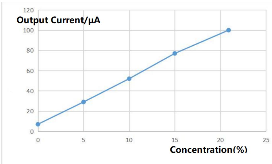
Here is the correlation between MIX8410 output current and concentration of O<sub>2</sub>. The current of 20% concentration O<sub>2</sub> is around 96uA. So the Grove SIGA voltage @ 20% concentration = R7 \* Current(MIX8410) \* 241 = 100 \* 96uA \* 241 = 2.314V.
