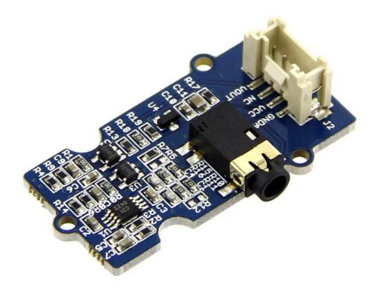
EMG detector is a bridge connects human body and electrical, the sensor gathers small muscle signal then process with 2th amplify and filter, the output signal can be recognized by Arduino. You can add this signal into your control system.
