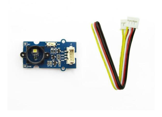
This module is based on the color sensor TCS3414CS with digital output I2C. Based on the 8\*2 array of filtered photodiodes and 16-bit analog-to-digital converters, you can measure the color chromaticity of ambient light or the color of objects. Of the 16 photodiodes, 4 have red filters, 4 have green filters, 4 have blue filters and 4 have no filter(clear). With the synchronization input pin, an external pulsed light source can provide precise synchronous conversion control.
