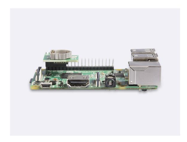
Please make sure plug the pin 1 of this hat into the pin 1 of raspberry GPIO, just like the picture above.
