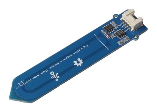
The Grove - Capacitive Moisture Sensor (Corrosion Resistant) is a soil moisture sensor based on capacitance changes. Compared with resistive sensors, capacitive sensors do not require direct exposure of the metal electrodes, which can significantly reduce the erosion of the electrodes. Hence, we call it **Corrosion Resistant**.
