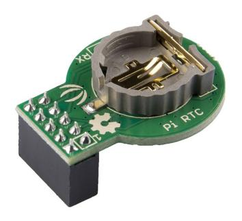
The Pi RTC is based on the clock chip DS1307, it can provide a real-time clock(RTC) for raspberry pi via the I2C interface. Real-time clock of this module counts seconds, minutes, hours, date of the month, month, day of the week, and year with leap-year compensation valid up to 2100. The clock operates in either the 24-
