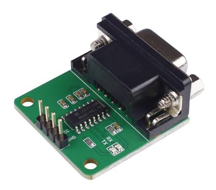
Most of the MCUs use TTL levels, and the computer serial port generally uses 232 levels. If we want the computer to communicate with the MCU, we need this **RS-232 To TTL Conveter** (MAX3232IDR).
