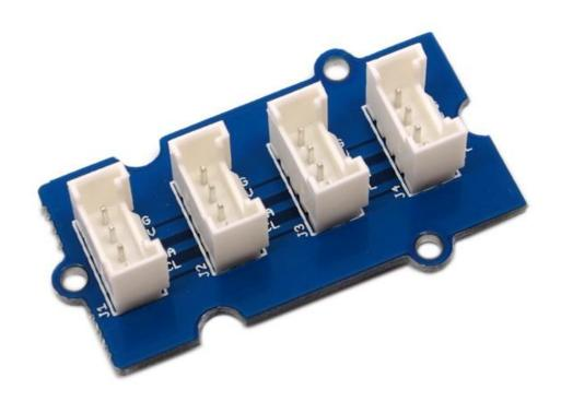
I2C Hub Grove is an extension Grove module for connecting multiply I2C devices to Grove Base Shield. It can use with Universal 4 Pin to X2 4 Pin cable
