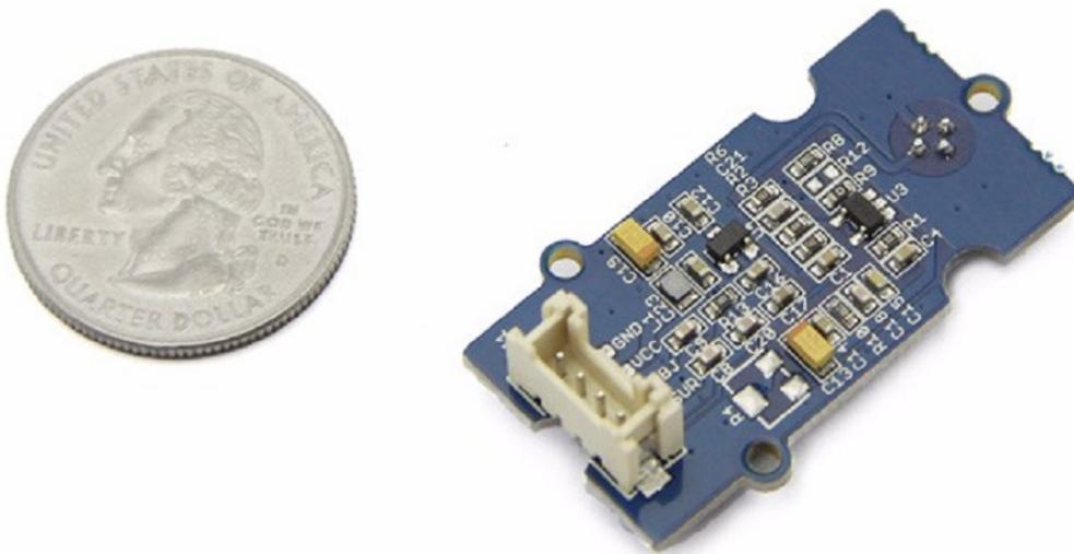
The Infrared temperature sensor is a non-contact temperature measure model. It is composed of 116 elements of thermocouple in series on a floating micro-membrane, the black Surface of the sensor is good to absorb the incident thermal infrared radiation, which might trigger a voltage response at output. This sensor outputs an analog voltage (0~1.1V) according to target temperature.
