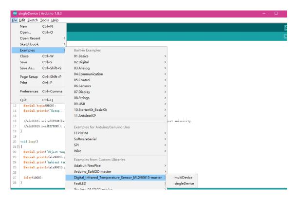
Since the sensor is factory calibrated with the digital SMBus compatible interface enabled, but the library is based on a soft i2c library, so you can use any digital pins on any AVR chip to drive the
