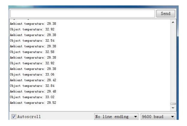
Now, you can measure the temperature with this sensor. Ambient temperature is the MLX90615 package temperature and Object temperature is the object target temperature. According to our experiment, when you place the sensor in the normal indoor temperature, and ensure that there is nothing source of heat in front of the sensor's 1M scope. The Object temperature will approximately equal to Ambient temperature. When measuring the
