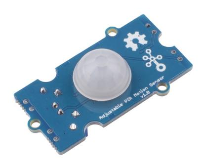
Grove - Adjustable PIR Motion Sensor is an easy to use Passive Infrared motion sensor, which can detect infrared object motion up to 3 meters. Any infrared object moves in its detecting range, the sensor outputs HIGH on its SIG pin. And you can adjust the SIG
