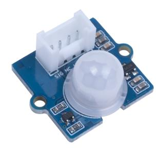
PIR sensor is an IR sensor to detect human motions. This Grove Digital PIR Sensor is the cheapest PIR sensor in the PIR families, however, it is able to give a quick response and generate a high signal from the "sig" Pin.
