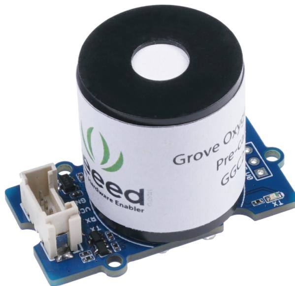
Grove - Oxygen Sensor Pro(GGC2330-O2) is a kind of sensor to test the oxygen concentration in air, which is based on the principle of the electrochemical cell to the original work. When it starts to work, it will produce a current proportional to the concentration of oxygen,
