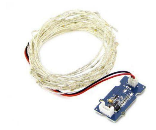
The Grove - LED String Light module is essentially an LED driver for the LED string lights included in the pack. Working voltage of the module is 3.3V/5V. However, the LED string lights require a working voltage of 12V. Therefore, this module uses a AIC1896 current mode step up DC-DC Converter to provide the requisite voltage to the LED string lights. The LED string light is 5 meters in length and
