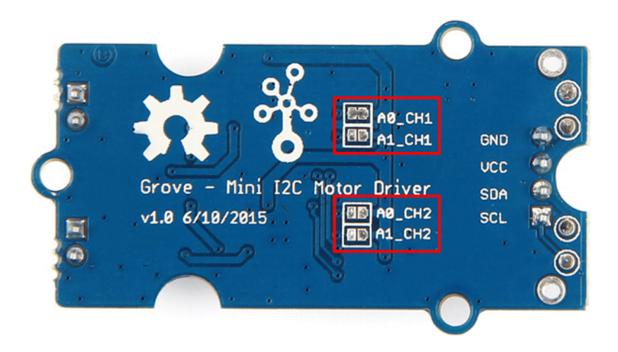
You can solder or unsolder each jumper to change the I2C address:
