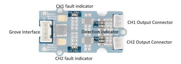
Grove Interface - Grove products have a eco system and all have a same connector which can plug onto the Base Shield.
