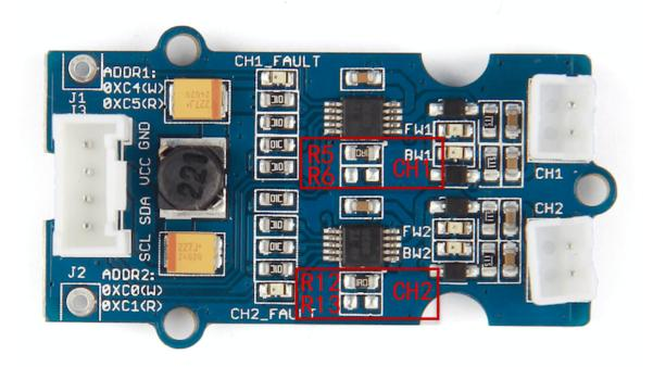
Each channel (CH1,CH2) has been added a resistor, and each value of resistor (R5,R12) is 1  $\Omega$ , so the maximum drive current is 200mA according to the following equation
