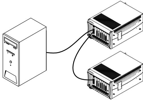
If you are using an embedded controller, you can use a PXIe-8394 to expand to additional chassis. As with a PC host, you can use a PXIe-8394 card per additional chassis (preferred), or you can daisy-chain additional chassis using the PXIe-8399. The PXIe-8394 backplane connection is limited to Gen 3 x8.
