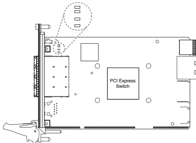
The Backplane Link Status LEDs report the status of the PCI Express links established between any PCI Express switches that reside on the backplane of the chassis that the PXIe-8398 or PXIe-8399 is controlling. In some cases, the link is with the peripheral boards installed in the chassis passive slots.
