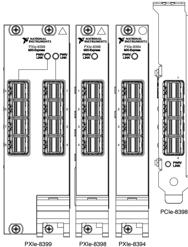
Port 1 of the PXIe-8398 and PXIe-8399 is upstream facing, meaning it is the link going toward the host. This means it is connected to a PXIe-8394, PCIe-8398, or a downstream facing port of a PXIe-8398 or PXIe-8399.
