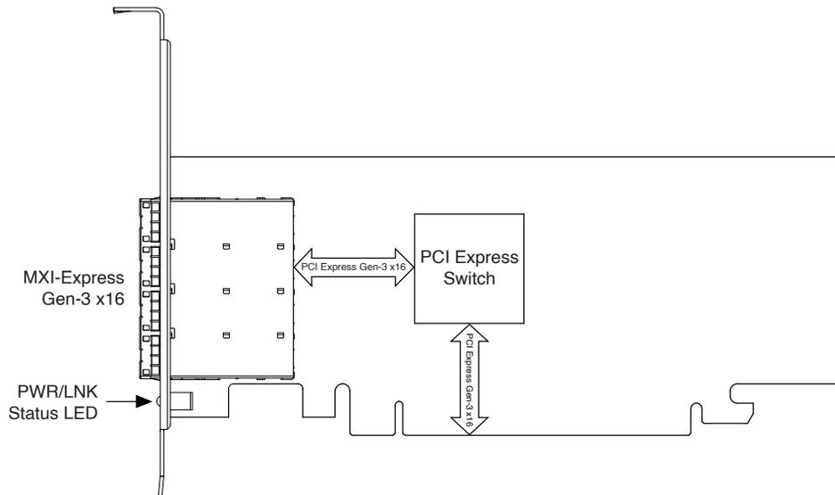
Figure 2. PXIe-8398 (156874x-01L) and PXIe-8399 (156874x-02L) Block Diagram
