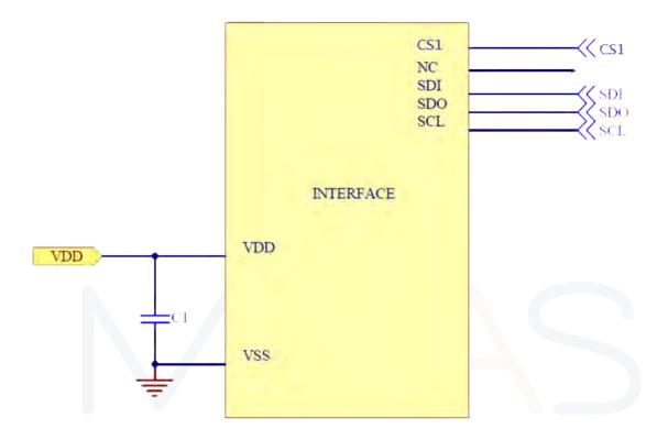
Pin connected to MCU interface: CS1,SDI, SDO, SCL
