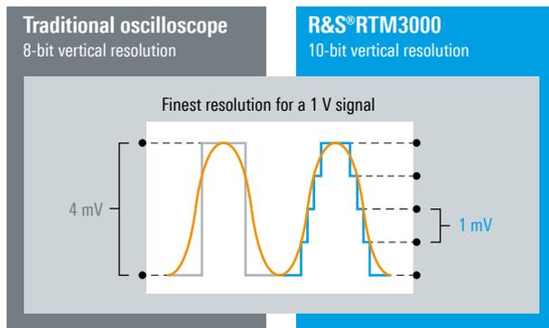
One example is the characterization of switched-mode power supplies. The voltages across the switching device must be determined during the on/off times within the same acquisition. For precise measurements of small voltage components, a high resolution of more than 8 bit is essential.
